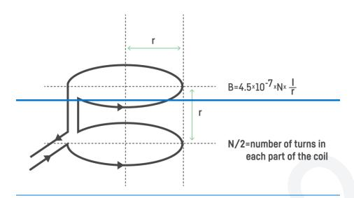
Figure 9.3.4.4. Calibration using a Helmholtz-type calibration coil.
