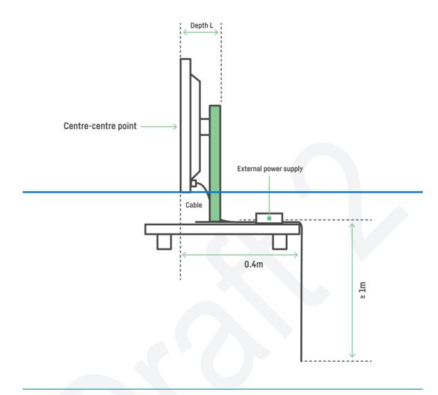
Figure 9.3.3.2. Display with external power supply units.
