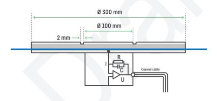
Figure 9.3.4.1. Sketch and circuit principle of the Alternating electric field meter for alternating electrical field measurements. The feedback circuit of the operational amplifier is a capacitance C in parallel with a high value resistor R to ensure that there is no DC voltage across the plates of the capacitor C.
