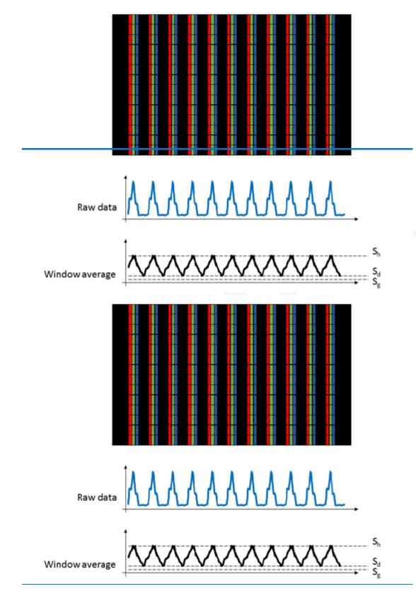
Figure *Luminance contrast - characters 1*: Measurement principle (from IDMS 7.2). In summary:
