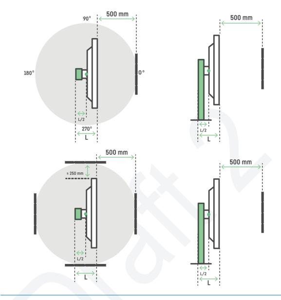
Figure *alternating electric fields 1*. Measurement geometry for band I (top) and band II (bottom).
